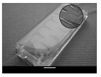
**Fig. 1** - Dual-layer microsystem in PDMS for tissue engineering of alveolar tissue. The close-up displays details of the microvascular network adjacent to the parenchymal compartment. Scale bar = 1 cm.
