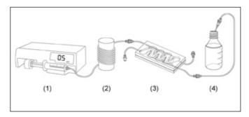
**Fig. 2** - Schematic representation of the dual-layer culture system in PDMS. Culture medium is delivered by a syringe pump (1) through silastic tubing via a custom-made oxygenator (2) to the vascular network in a microfabricated dual-layer microsystem (3). It provides separate inlets and outlets for the vascular compartment and the parenchymal compartment. The effluent is collected in a waste container (4).
